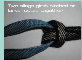
Two slings strop hitched together
